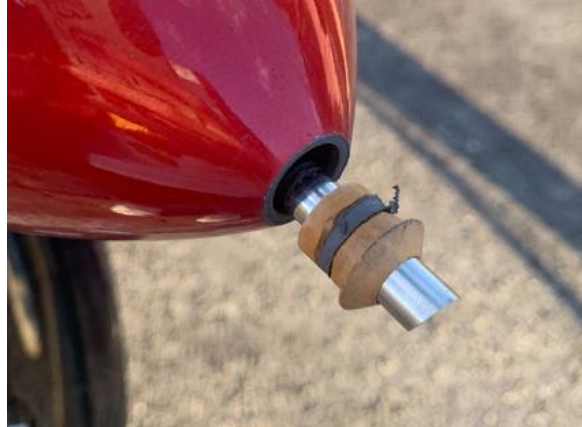
FIGURE 1: ADHESIVE FAILURE EXAMPLE
