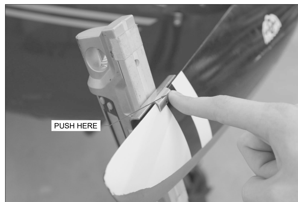
FIGURE 3: SEATING THE PROP PITCH BRACKET
