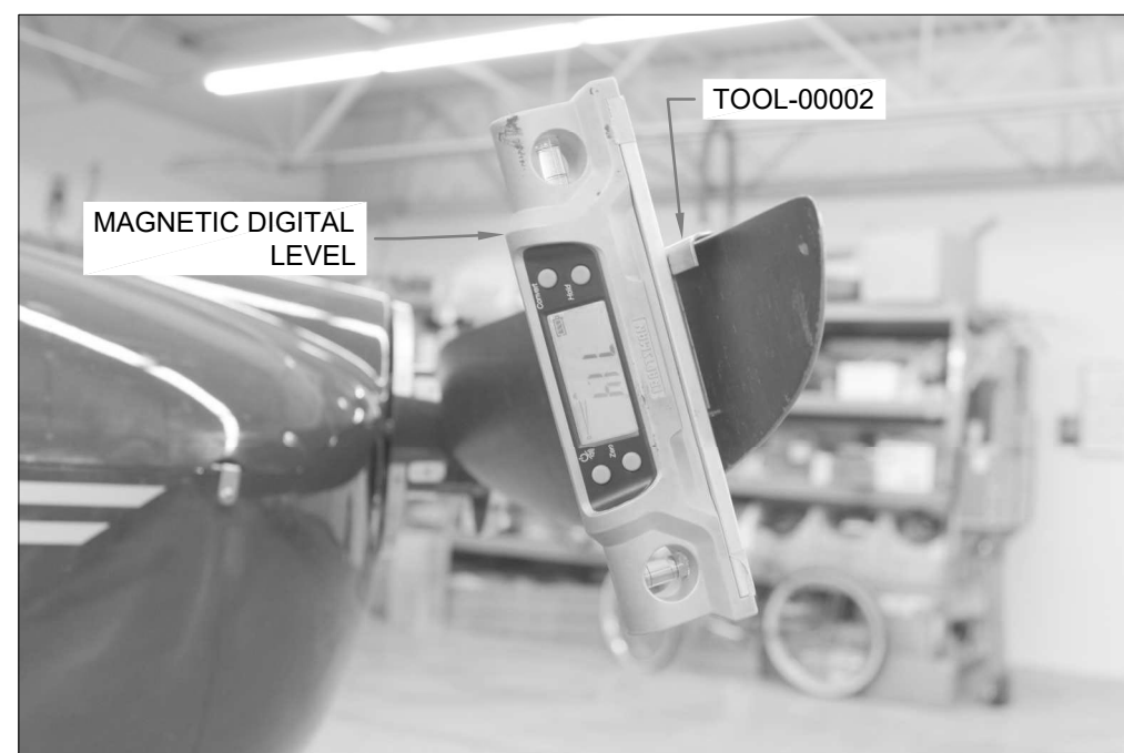
FIGURE 1: MEASURING THE PITCH ANGLE
