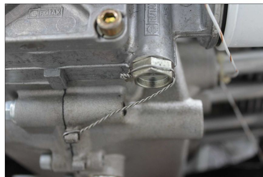
FIGURE 4: SAFETY WIRE OIL PRESSURE REGULATOR PLUG
