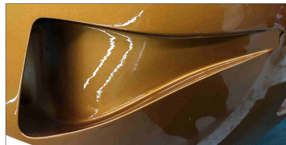
FIGURE 3: FINISHED ENGINE AIR INLET
