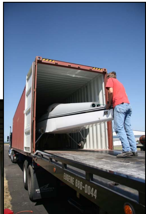
Two RV-6As leave the USA for Sweden. Disassembly and containerizing was taken accomplished at SynergyAir in Eugene, OR.. The special stamp on the wood crate shows that it was built from wood acceptable for international shipment.
