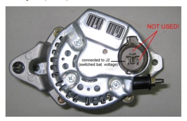
There is a three terminal plug on the back of the alternator. When viewed from the back with the two parallel terminals down, only the lower left terminal should be used. This will normally correlate to the green wire on the plug. The other two terminals (red and blue wires) are not to be used. Please see the diagram on page 2.
