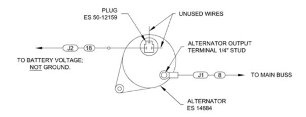
If your alternator is currently wired to the old configuration, all you need to do is remove the connection for the red wire. Older alternators will also function correctly with only the green wire connected.
