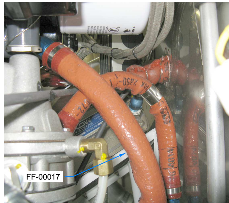
FIGURE 3: HOSE ROUTING (TAIL DRAGGER - LEFT SIDE VIEW)
