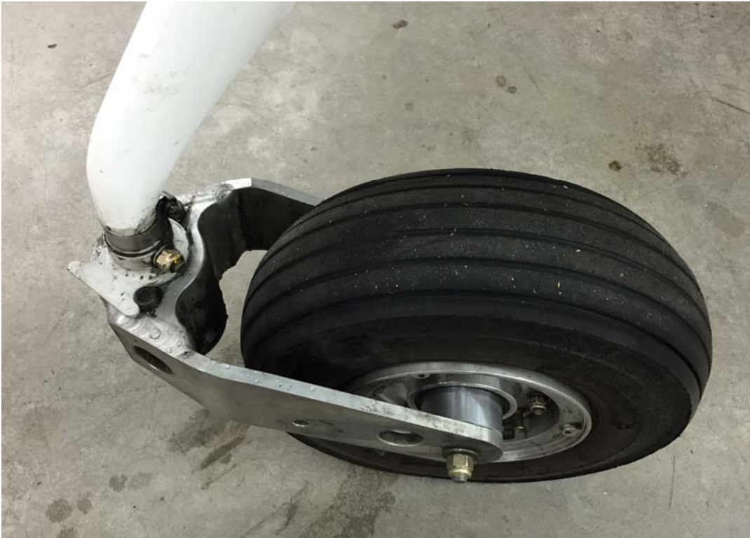
FIGURE 2: Nose Stop Flange Correctly Installed (Full Right Turn)
