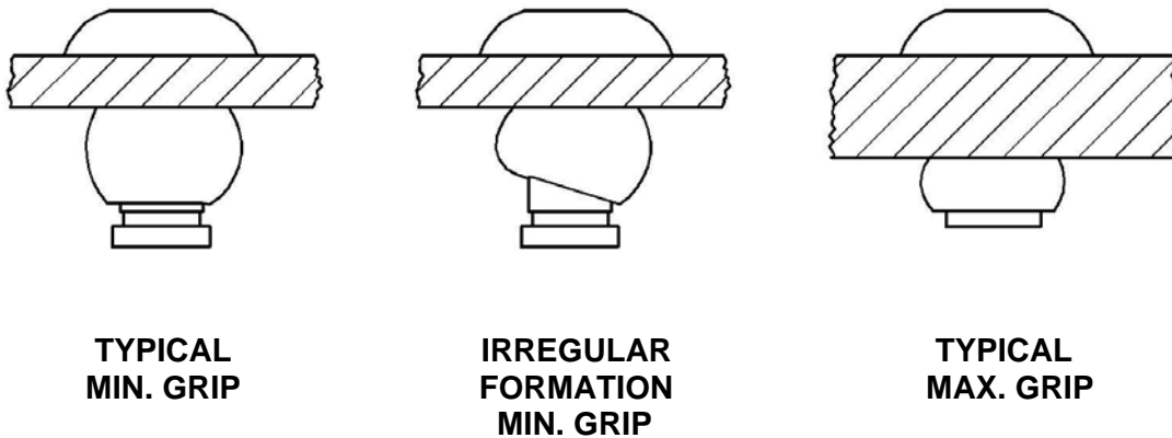
FIGURE 14D: ACCEPTABLE BLIND HEAD FORMATIONS.
