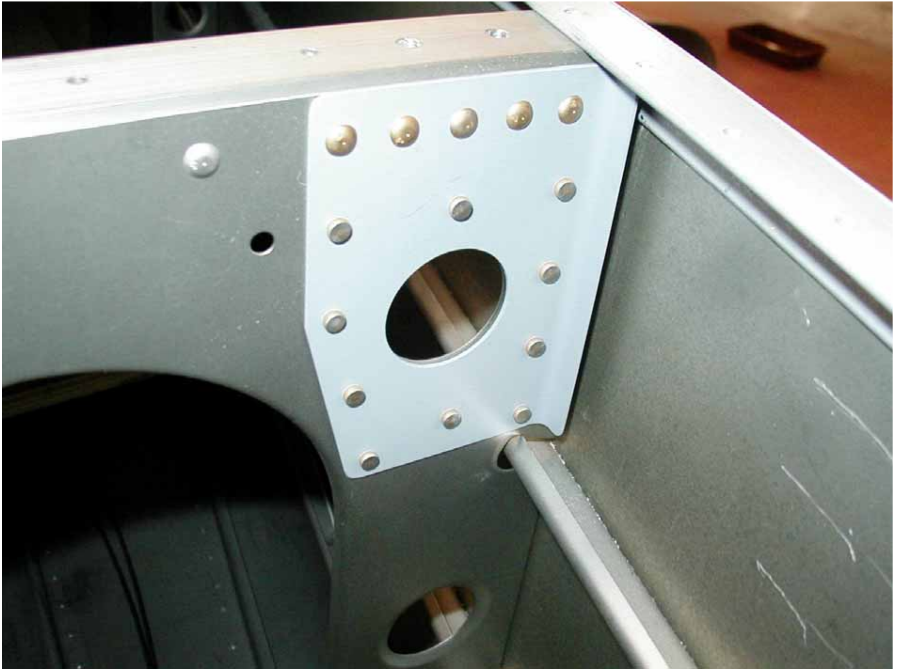
F-1010C doubler riveted in place.
