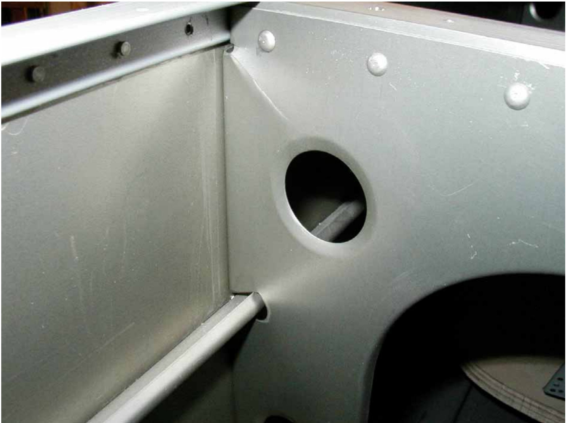
Crack in the upper left corner of F-1010 bulkhead....as seen from the back side looking forward.
