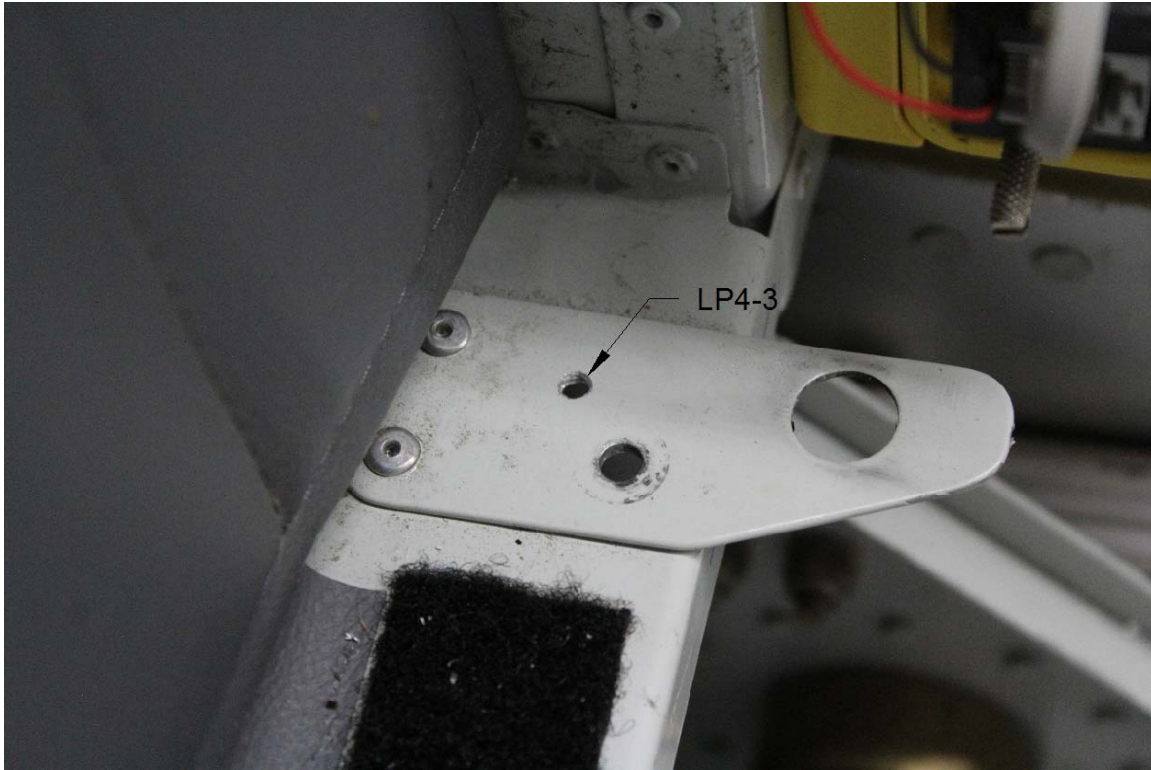
FIGURE 4: NEW RIVET LOCATION
